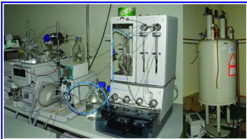
Figure 1. Photo of the HPLC–SPE–NMR (400 MHz) in School of Pharmacy, College of Medicine, National Taiwan University. (Photo taken by SS Lee.)
